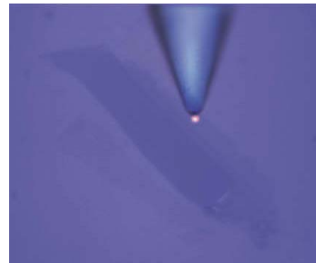
White light image of the graphene flake with AFM tip and Raman laser
