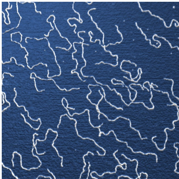
Figure 1: Linearized Plasmid DNA (pGem7zf+ from Promega) adsorbed onto muscovite mica. Image scan area corresponds to 2\ \mu\text{m} \times 2\ \mu\text{m} .
