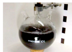
Fig 4: A stirred 10 liter reaction vessel with 1 g of suspended TurboBeads (left). The 30 nm metal nanobeads can be separated from the liquid with a commercial low-cost magnet (right; left side of the vessel) within just 5 minutes.
