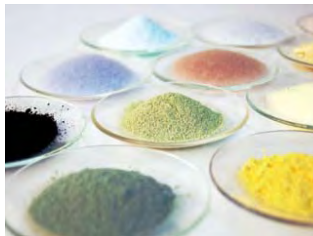
Figure 1. Using flame spray synthesis, the compositional variety of inorganic nanoparticles is nearly endless. Different oxidic, salt and metallic nanoparticles with similar particle size distribution are depicted (courtesy of Nanograde LLC.).
