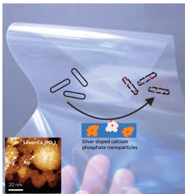
Figure 3. Composite nanoparticles with 1-2 nm silver nanoparticles homogeneously distributed on calcium phosphate carrier nanoparticles. Due to the small size and distribution on the surface of salt nanoparticles, these nanocomposites are up to 1000 times more efficient bacteria killers than conventional silver preparations.
