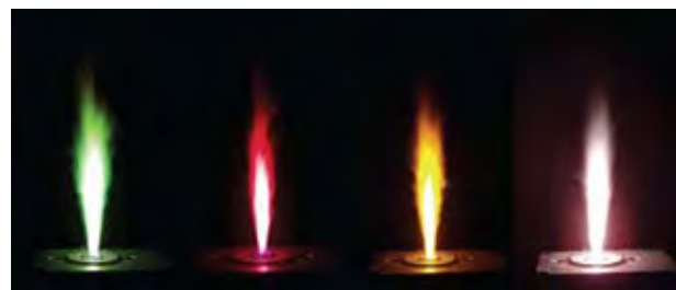
Figure 2. Depending on the metal loading the flames during the production of inorganic nanoparticles show different colors. Illustrated in this example is the combustion of metalorganic precursors containing copper, strontium, cerium and bismuth (from left to right).
