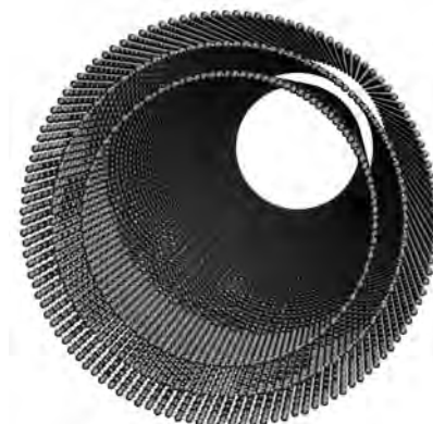
Figure 3.1b Schematic of a multi-walled carbon nanotube (MWNT)
