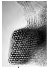
Bundle of single-walled carbon nanotubes (approximately 1.4 nm wide, several mm long) A. Thess et al., Science 273, 483, 1996
