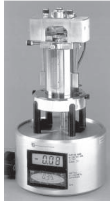
Measuring head of an atomic force microscope
