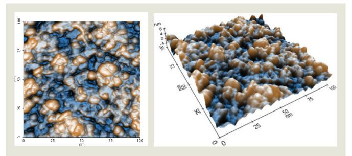
Figure 2. High resolution (100 nm x 100 nm) image of a gold surface, acquired by True Non-Contact Mode of the XE-100 AFM.
