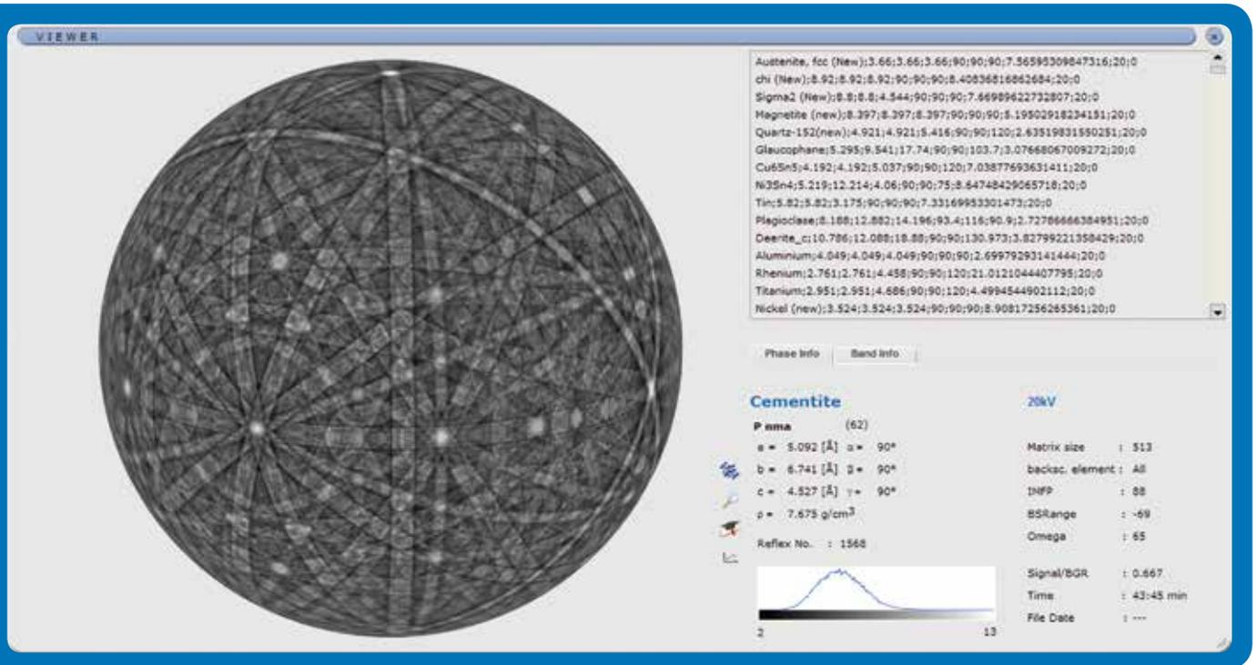
Viewer for simulated EBSD patterns showing the projection on a sphere for cementite. A double click on the sphere will change the display to gnomonic projection, equivalent to experimental patterns.
