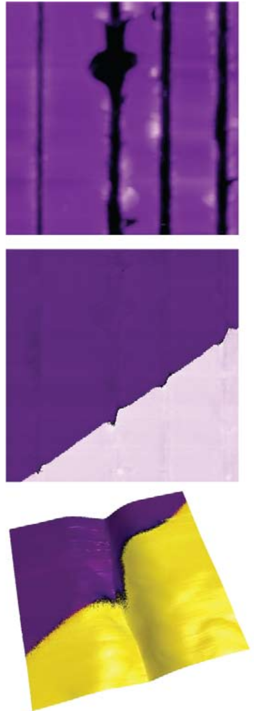
Figure 32: Surface topography of PPLN after it has been purposefully scratched with different loading forces using the NanoIndenter, 10µm scan (top and middle images). 1µm scan (bottom).
