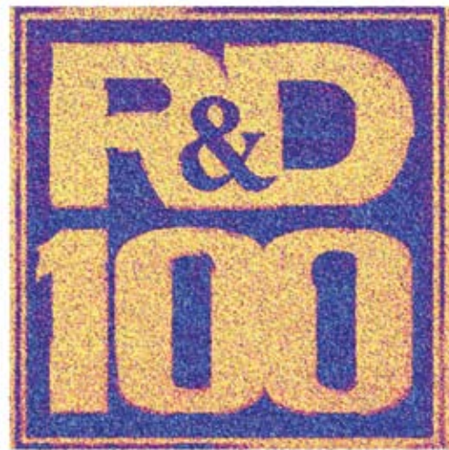
Figure 7: R&D 100 logo written on a sol-gel PZT thin film by PFM lithography. PFM phase is overlaid on top of the rendered topography, 25μm scan. Oak Ridge and Asylum Research were awarded an R&D100 award for Band Excitation in 2008.
