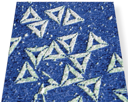
DNA origami triangles , imaged in fluid, ~120 nm per edge, 600 nm scan. Sample courtesy of P.W.K. Rothemund, California Institute of Technology.
