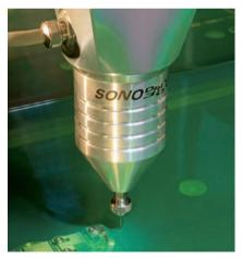
Vibrations of a piezo actuator reduce the processing times for high-precision micro-sized holes (image: ICT-IMM)
