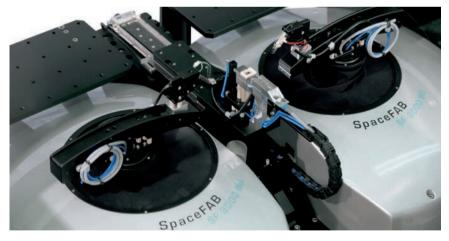
Alignment of optical fibers on a microchip in 6 axes
