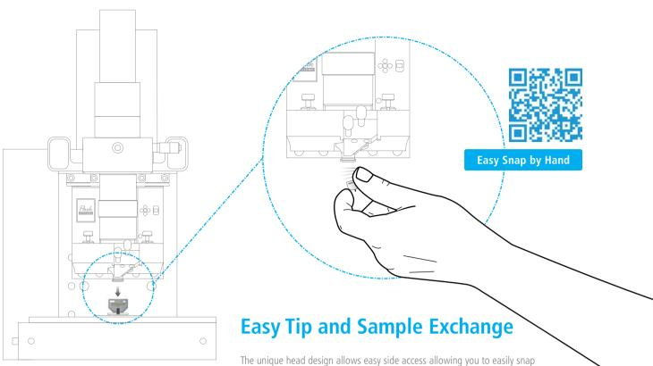
The unique head design allows easy side access allowing you to easily snap new tips and samples into place by hand. The cantilever is ready for scanning without the need for any tricky laser beam alignment by using pre-aligned cantilevers mounted on to the cantilever tip holder.
