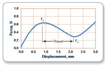
Figure 5. Force-displacement of a keyboard obtained using DFM-0.5 and a LVDT sensor.
