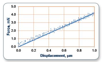
Figure 1. Force-displacement plots up to 5 mN using a Gold series FL sensor and Cap sensor.
