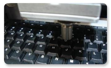
Figure 4. Close-up view of the test setup for force-displacement measurements on a keyboard.
