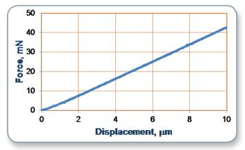
Figure 2. Force-displacement plots up to 50 mN using a Gold series FL sensor and Cap sensor.
