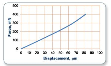
Figure 3. Force-displacement plots up to 400 mN using a Gold series FL sensor and Cap sensor.
