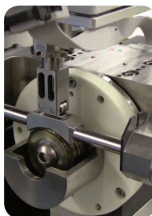
Figure 12. Lower drive and modules for lubricant test: (a) Rotary Module, (b) Linear-Reciprocating Module, (c) Block-on-Ring Module, and (d) 4-Ball Module.
