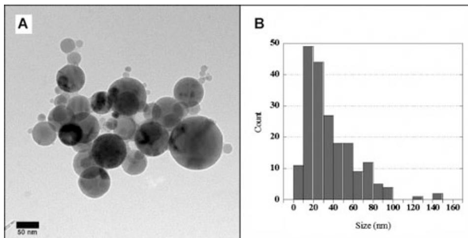
(A) Transmission electron microscopy (TEM) images of commercial aluminum oxide nanoparticles. (B) Size distribution obtained from TEM images.
