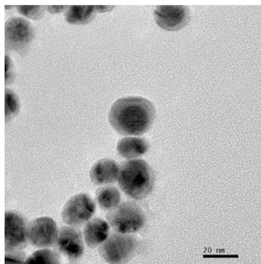
*Representative TEM image of core-shell nanoparticles prepared using a mixture of formaldehyde and ascorbic acid.*
